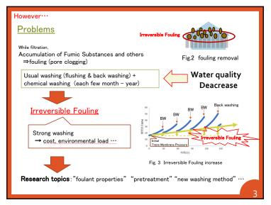
Membrane Filtration Membrane **pore** size with 10 nm $\sim$ 1  $\mu$  m. Removal of particles from water (solution) on the basis of size. advantage increasing easy Eco-friendly Maintenance - rural water system Space - Urban/Industrial water universal Use saving 1999 2001 2003 2005 2007 2009 2011 2013 2015 2017 Fig. 1 Share of membrane (水環境学会誌2021、2月号特集) 図4 全浄水量に占める製ろ過浄水量のシェア
